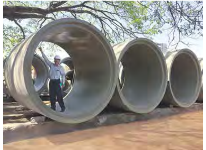
2600 mm dia RCC NP3 class pipes for Bangalore Water Supply & Sewerage Board, in Karnataka
