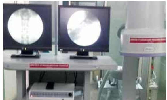
Allengers HF - 49R / PS 100 High Frequency (40 KHZ) Mobile C-ARM with accessories used in Orthopedic Department in Government Kilpauk Medical College, Chennai, Tamilnadu
