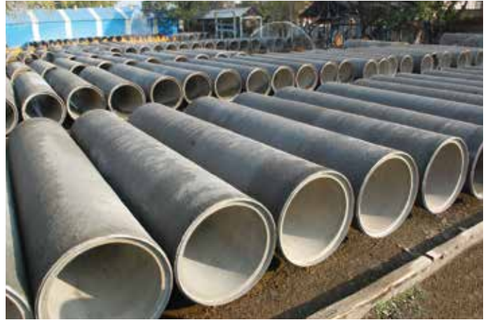
1200 mm dia PCC Pipe manufactured at Miraj factory, for Tillari Water Supply Scheme, Maharashtra
