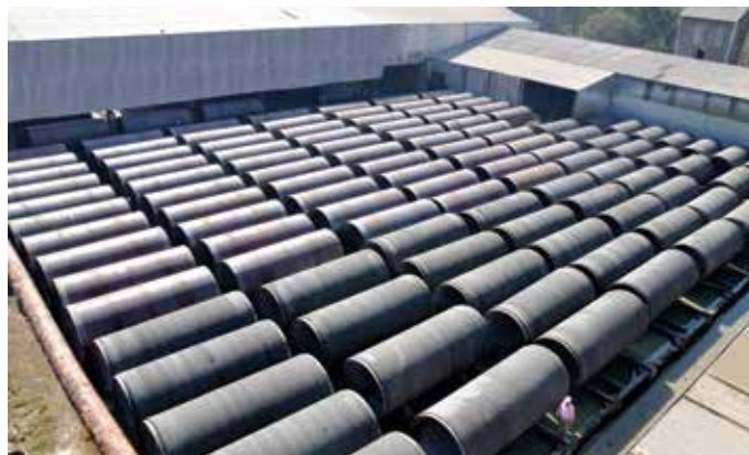
2200 mm dia MS pipe manufactured at Patancheru factory for Krishna Drinking Water Supply Project Package-IV Phase-III, Telangana.
