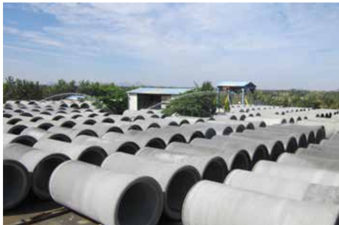
1900 mm dia PSC Pipes manufactured at Chilamathur Factory for Pulakurthy Lift Irrigation Scheme, Andhra Pradesh
